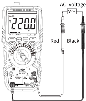
Wiring diagram when voltage is less than 1000V
