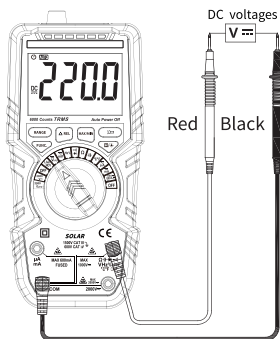
Wiring diagram when voltage is less than 1000V
