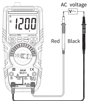
Wiring diagram when voltage is above 1000V
